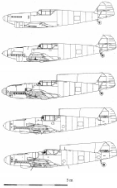
Fig. 3. The prototype and some versions of Messerschmitt Bf 109 from top to bottom: V1, A-1, E-1, F-1 (NE+ML) and G-6 (MT-507). Drawings by Klaus Niska.
