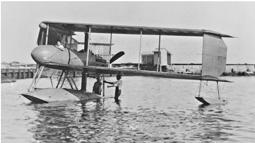
An American Burgess-Dunne AH-7 Flying Wing trainer at Pensacola Naval Air Station circa 1916. Though pleasant to fly, the Burgess-Dunne designs in Navy (and Army) service did not enjoy great success and were replaced by more conventional biplane designs. (Naval History and Heritage Command)
