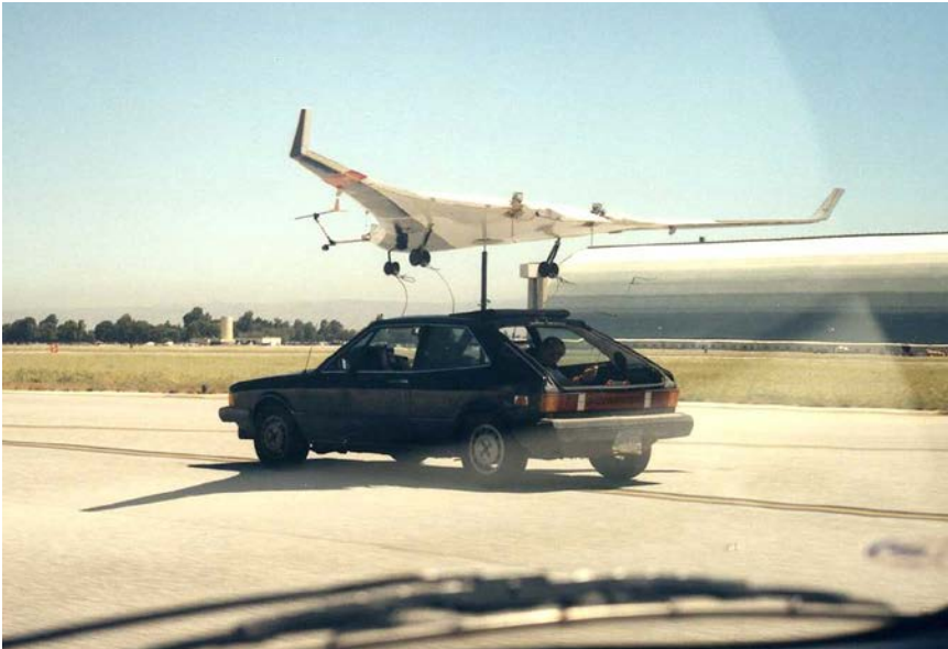
The BWB-17 during a high-speed road test at NASA Ames Research Center, Moffett Federal Airfield, CA. Behind the vehicle is Moffett's signature airship hangar, a skyline fixture since the days of the great naval airships in the 1930s. (Photo courtesy of Blaine Rawdon)
