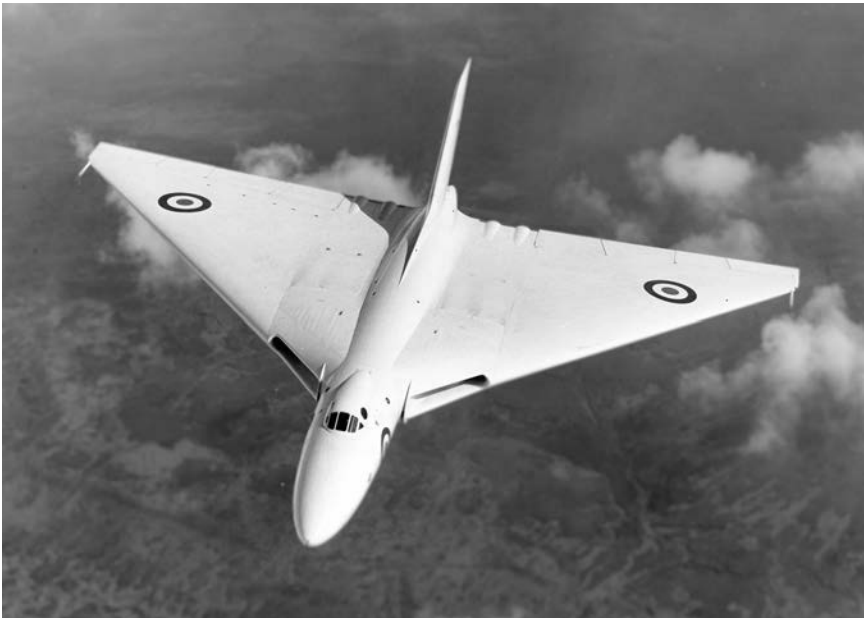
The Avro Vulcan, a four-engine delta-winged strategic bomber, represented a very different design approach—and, for its time, equally radical—to long-range strategic bomber design from Boeing's B-47. (National Museum of the United States Air Force [NMUSAF])
