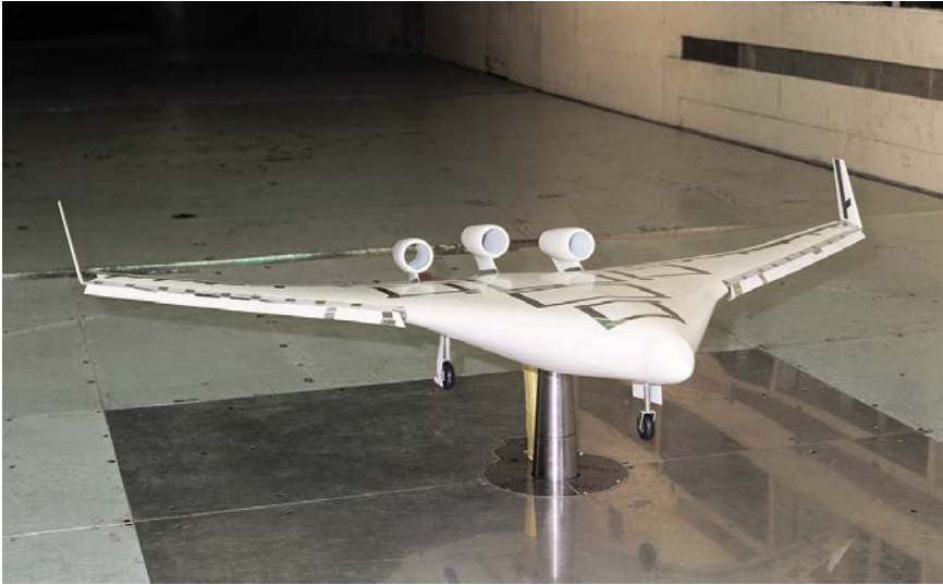
The 3-percent BWB model in the Langley 14- by 22-Foot Tunnel, with leading-edge slats extended and landing gear down. (NASA)
