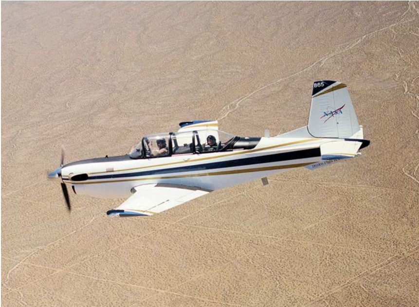
NASA 865, the two-place Beech T-34C Turbo-Mentor trainer, used by Dryden as a general mission support airplane, proved an ideal chase aircraft for the X-48B/C. Here it is flying over the Mojave on June 20, 2005. (NASA)
