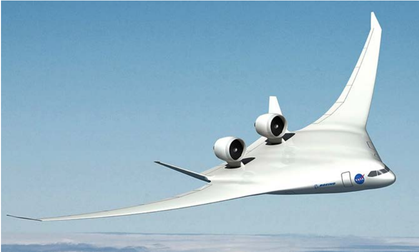
Boeing's Hybrid Wing-Body (HWB) transport concept submitted in response to NASA's Environmentally Responsible Aviation project. (NASA)
