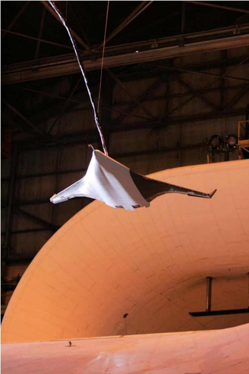
A 5-percent scale free-flight model of the BWB-450-1L configuration “flying” in the historic NASA Langley Research Center Full-Scale Tunnel. (NASA)
