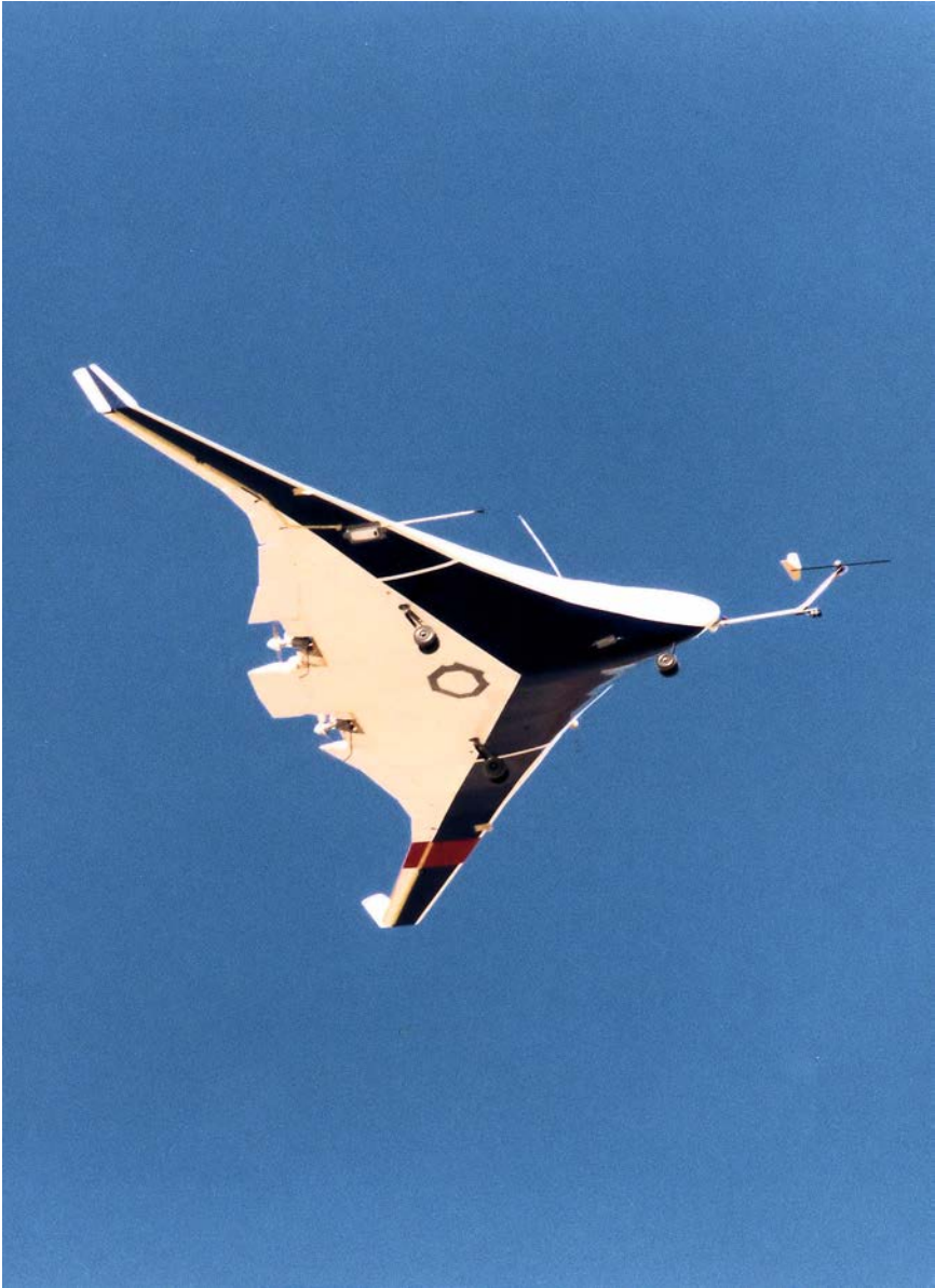
The BWB-17 in flight. Model tests with this aircraft and its predecessors played a crucial role in giving developers confidence to proceed with the X-48 development program. (Photo courtesy of Blaine Rawdon)
