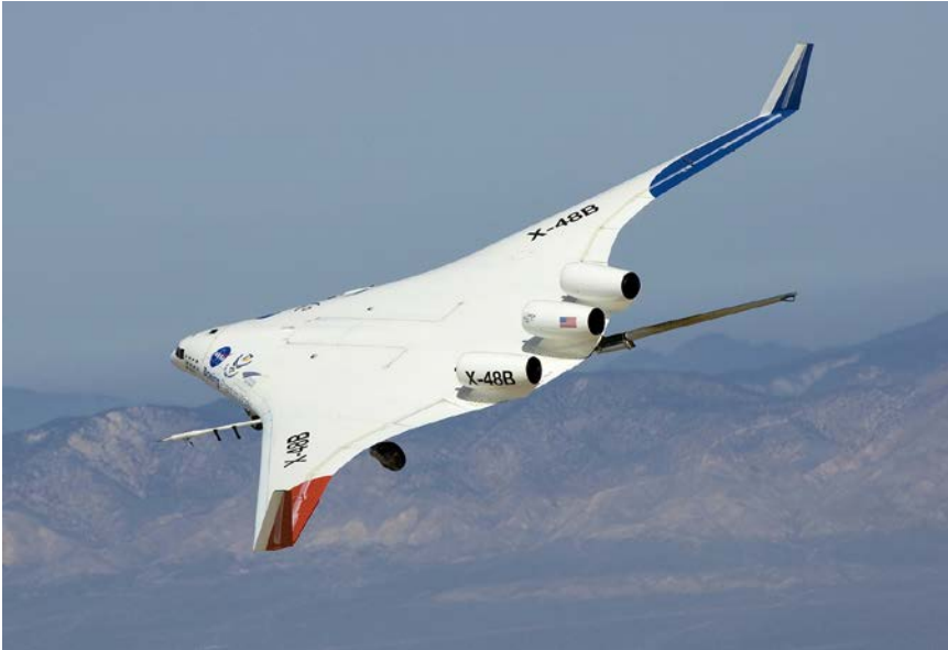
Piloted by Boeing’s Michael Sizoo, the X-48B banks gracefully on its 12th research mission, a 33-minute flight and the first with the BWB in the “clean wing” (i.e., with slats retracted) configuration. (NASA)
