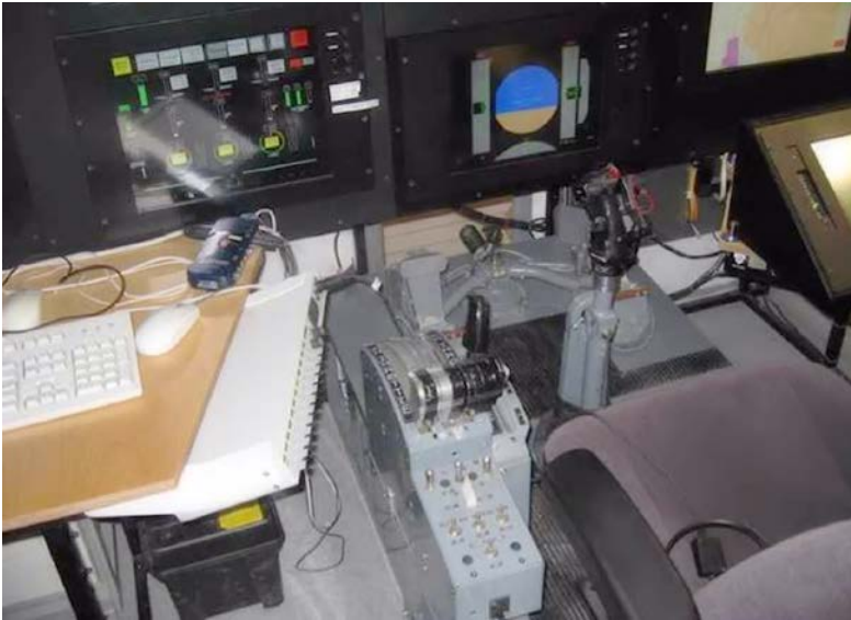
The X-48B's pilot position. Note that among the instrumentation and presentations, the pilot used a conventional control stick and left-hand throttle arrangement, with rudder pedals and a "head down" electronic artificial horizon display. (NASA)
