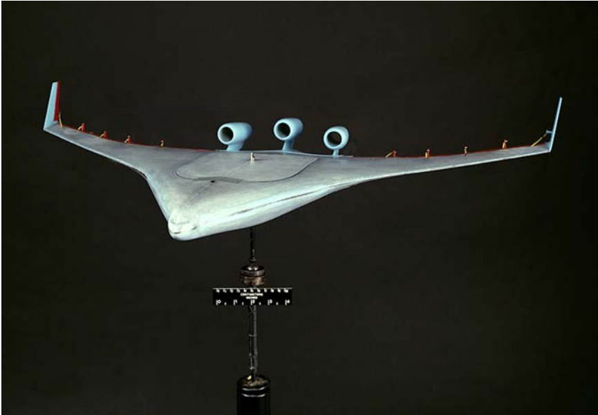
The 1-percent BWB-450-1L spin-test model being evaluated in the NASA Langley Spin Tunnel. (NASA)
