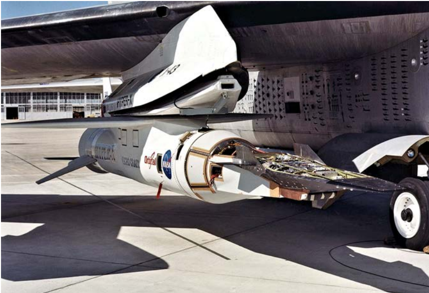
The ill-fated first X-43A Hyper-X launch stack under its NB-52B at Dryden in March 2001. Note the small Micro Craft X-43A scramjet test vehicle and the large modified Orbital Pegasus booster. The right elevon that separated is visible at the rear of the booster. (NASA)
