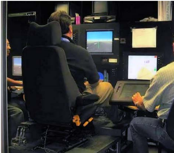
The X-48B Ground Control Station during a research mission. Note that the pilot is using the head-up display with video generated by the vehicle's nose camera. The head-down display is just visible above the pilot's right knee; the range safety officer is at the extreme left of the photograph; and the mission flight test engineer is at the right. (NASA)
