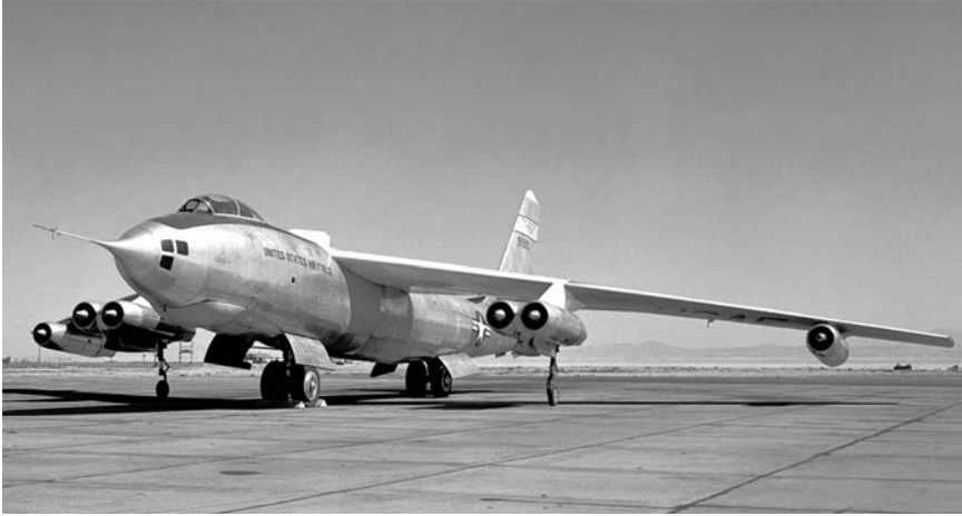
The first production Boeing B-47A Stratojet (SN 49-1900) while on loan to the National Advisory Committee for Aeronautics (NACA) High-Speed Flight Station, Edwards Air Force Base (AFB), CA, for comparative flight trials, in September 1953. Note the six podded jet engines, quickly adopted for large long-range sweptwing jet airliners such as Boeing's 707 and Douglas' DC-8. (NASA)
