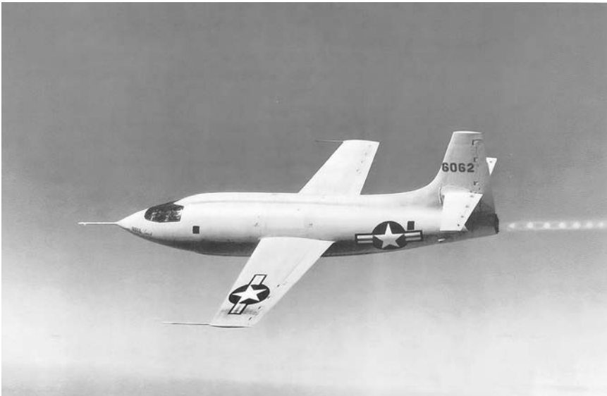
The Bell XS-1 (later X-1) no. 1 (SN 46-062) on its historic flight through Mach 1 on October 14, 1947, piloted by Capt. Charles E. “Chuck” Yeager. The air-launched XS-1 had a bullet-inspired shape, thin wings and tail surfaces, a modest aspect ratio, an adjustable horizontal tail, and rocket propulsion. (USAF)
