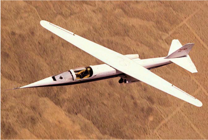
The diminutive Ames-Dryden AD-1 Oblique Wing Testbed (NASA 805) demonstrating controlled flight at 60-degree wing sweep during a 1980 research mission. (NASA)
