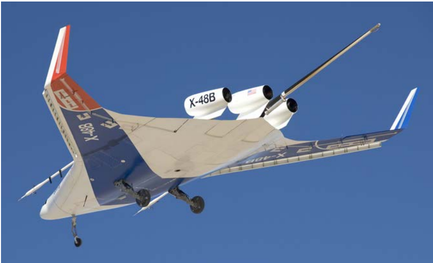
The X-48B shows its unique profile in this left ventral rear-quarter photograph; note the extended wing slats. (NASA)
