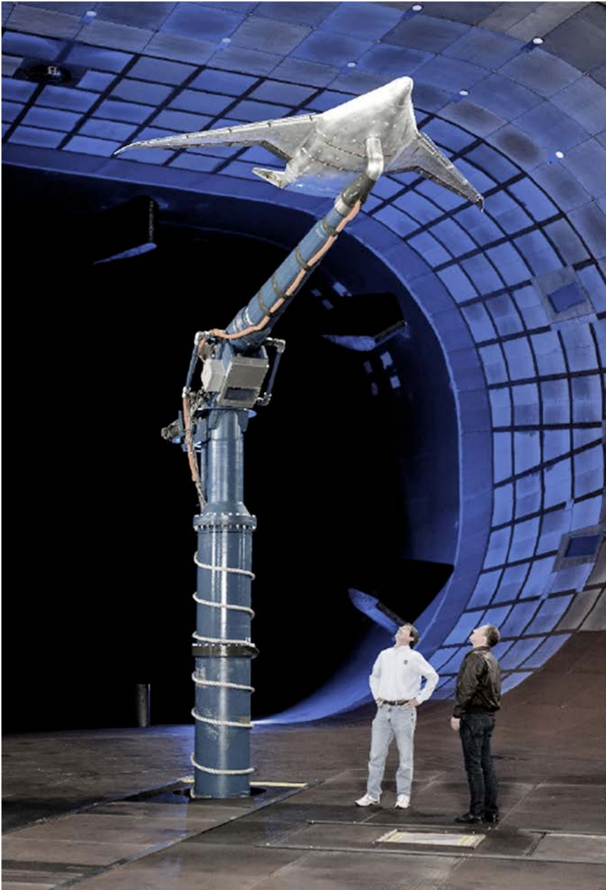
Readying a Boeing Hybrid Wing-Body for tests in Ames Research Center's 40- by 80-Foot National Full-Scale Aerodynamics Complex (NFAC). (NASA)
