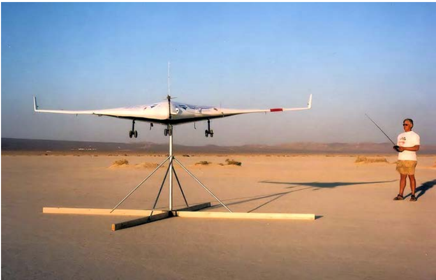
In preparation for the BWB-17’s first flight, pilot Bill Watson assessed the radio control and control surface function with the BWB-17 mounted on a pole at El Mirage Dry Lake, CA. (Photo courtesy of Blaine Rawdon)
