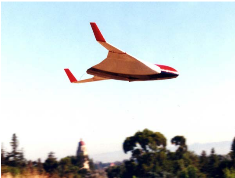
Stanford's initial BWB flight-test work was with this deceptively simple BWB glider. (Photo courtesy of Blaine Rawdon)
