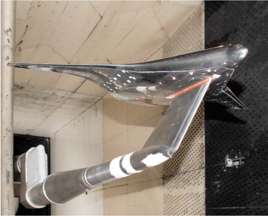
A 2-percent BWB-450-1L model tested in the Arnold Engineering Development Center's 16-Foot Transonic Wind Tunnel, Tullahoma, TN. (USAF)
