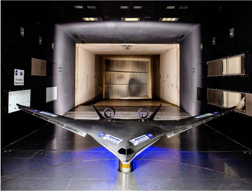
The 6-percent Boeing BWB undergoes testing in Langley Research Center's 14- by 22-foot Subsonic Tunnel in 2016. (NASA)
