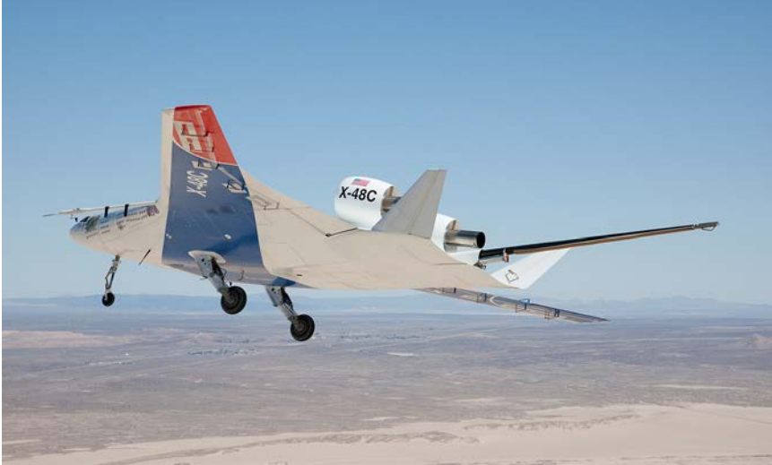
The X-48C banks over the northern lake shore of Rogers Dry Lake; note the clean wing (slats retracted) configuration. (NASA)
