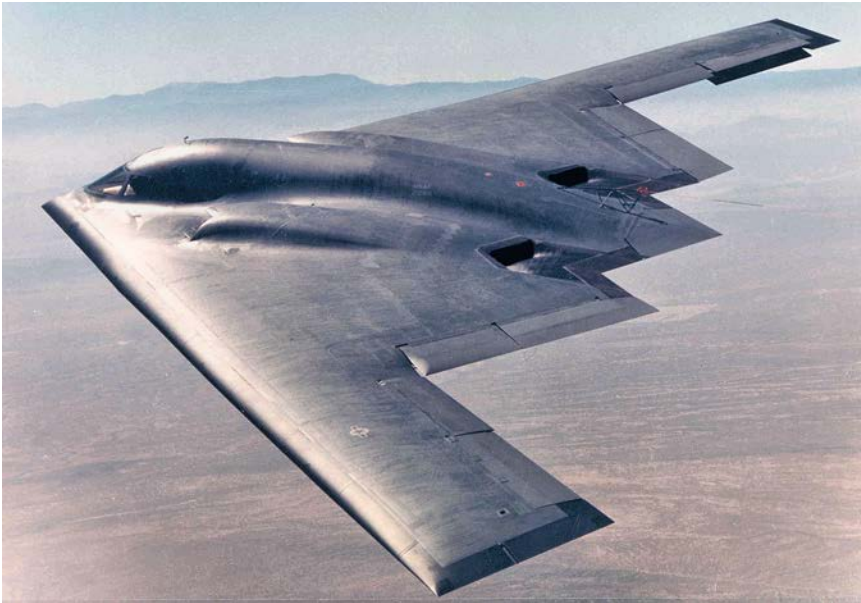
The first Northrop B-2A Spirit stealth bomber (SN 82-1066), whose first flight in 1989 heralded the age of the practical transonic flying wing. (USAF)
