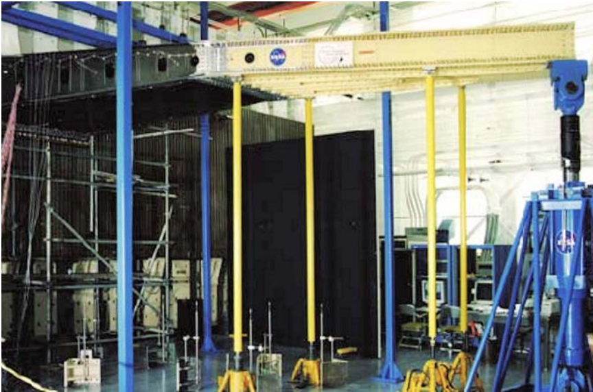
The McDonnell Douglas-fabricated composite wing stub box undergoing loads testing at LaRC in 1995. McDonnell Douglas subsequently merged with Boeing in August 1997. (NASA)
