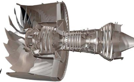
Advanced Core for UHB Turbofan (P&W GTF)
