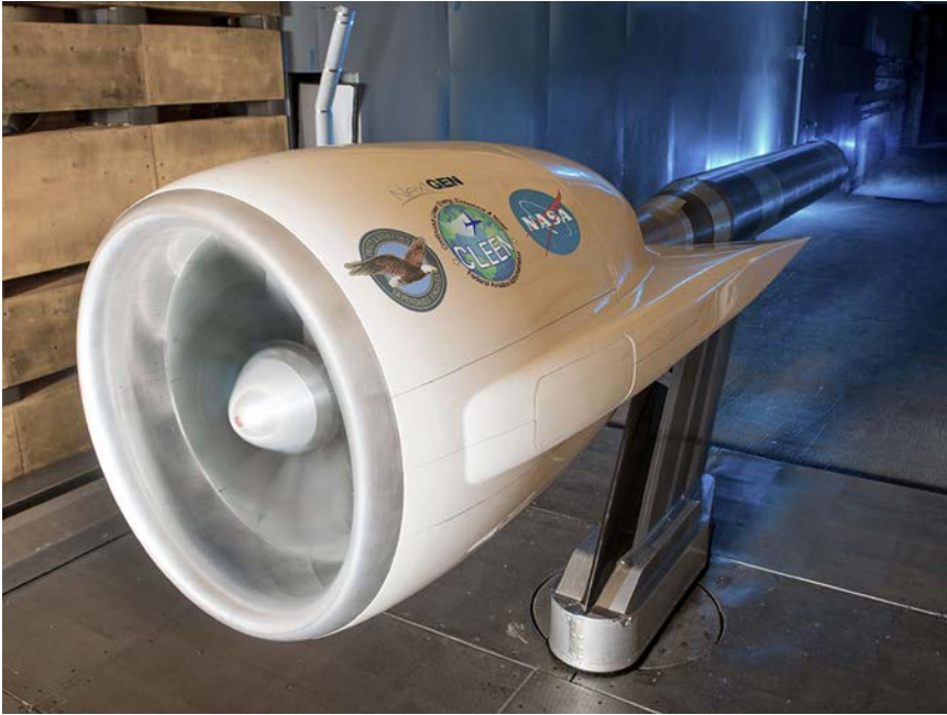
A Pratt & Whitney next-generation ultra-high-bypass-ratio turbofan model undergoing testing in the NASA Glenn Research Center's 9-by-15-foot Low Speed Wind Tunnel. (NASA)
