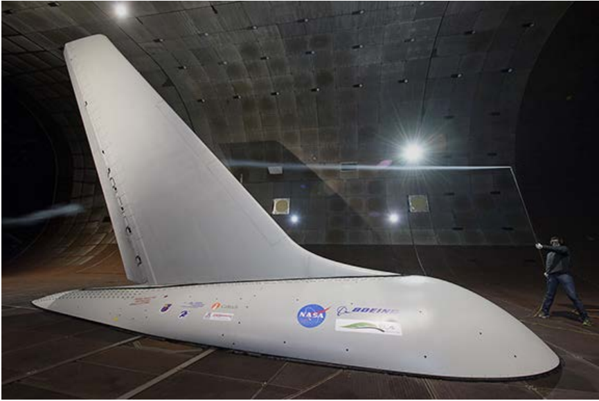
The Active Flow Control system was tested on a full-sized tail in the National Full-Scale Aerodynamics Complex (NFAC). (NASA)
