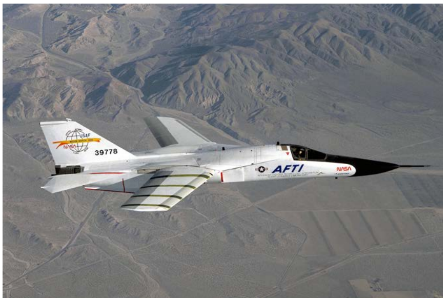
The Air Force-NASA AFTI F-111A (SN 63-9778) Mission Adaptive Wing (MAW) testbed on one of its test flights. (NASA)
