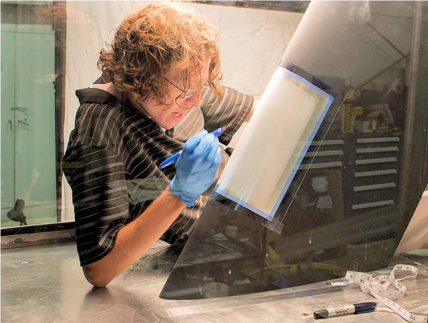
“Bug team” researcher John Gardner lies inside Langley’s Basic Aerodynamics Research Tunnel, or BART, to prep the leading edge of a scale model wing for a blast of bugs from the tunnel’s “bug gun.” (NASA)
