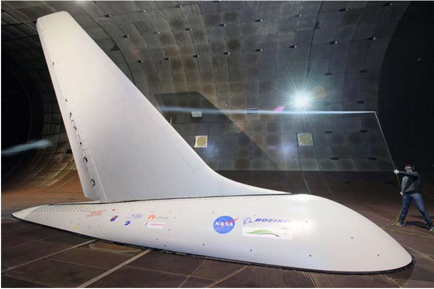
The Active Flow Control system was tested on a full-sized tail in the NFAC. (NASA)
