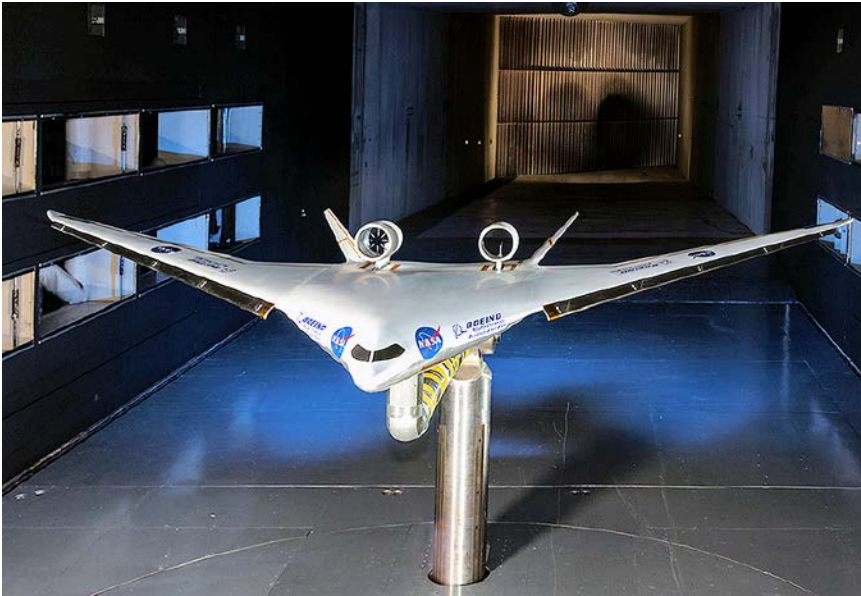
A Boeing HWB model in the 14-by-22-foot subsonic wind tunnel at NASA Langley Research Center. (NASA)
