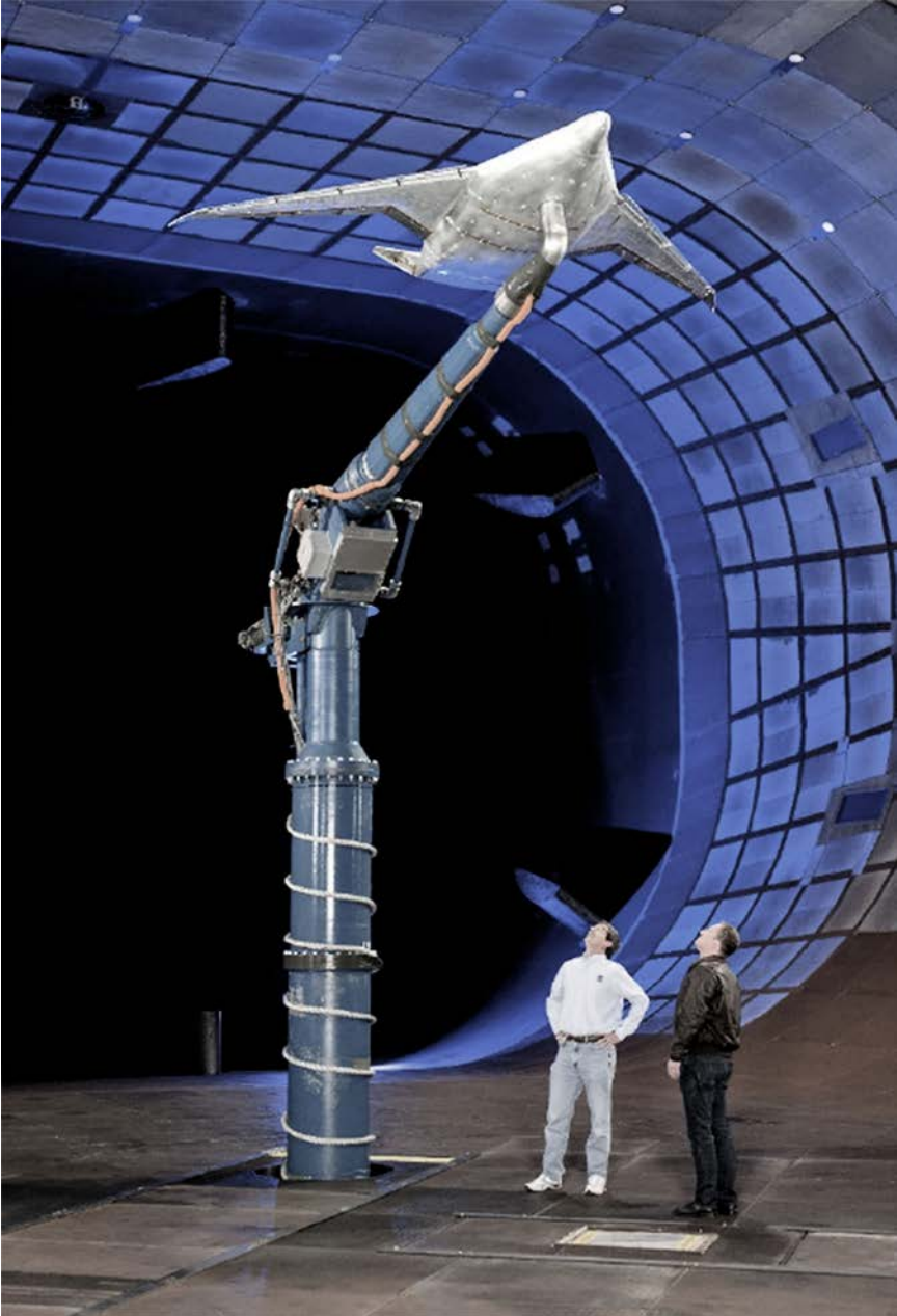
National Full-Scale Aerodynamics Complex (NFAC) 40-by-80-foot test section with a Boeing HWB model. The size of the NASA personnel gives a sense of the immense size of this now-70-year-old facility. (NASA)
