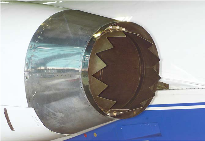
The distinctive saw-tooth engine chevron, an imaginative effort to reduce engine noise. (NASA)
