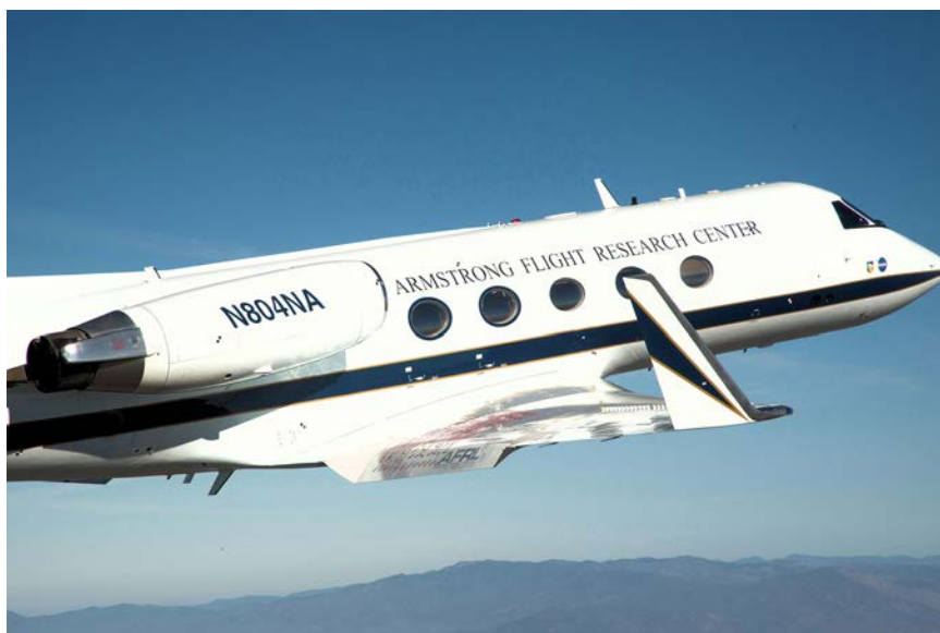
Flight test of ACTE flap at 25 degrees deflection. (NASA)
