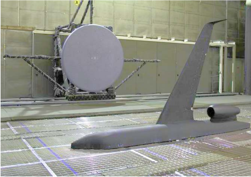
Test setup in the LaRC 14-by-22-foot wind tunnel with the 18-percent-scale semi-span G550 model and microphone array. (NASA)
