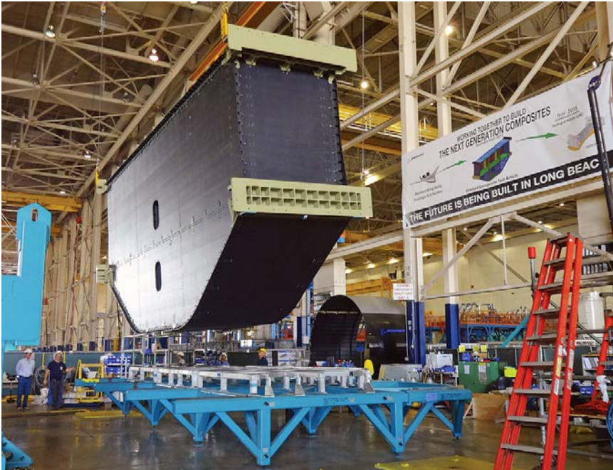
Following completion at Boeing's Long Beach facility, the PRSEUS MBB is prepared for shipment to LaRC. (NASA)
