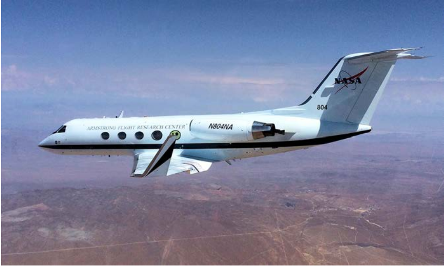
NASA's SCRAMjet testbed in flight. Note ACTE flap deflection. (NASA)
