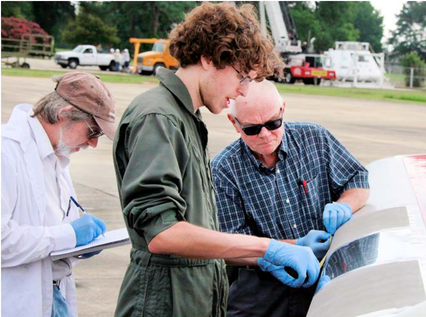
NASA researchers check results following preliminary flight tests of nonstick anti-insect coatings. (NASA)
