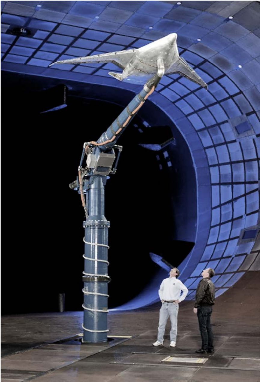
National Full-Scale Aerodynamics Complex (NFAC) 40-by-80-foot test section with a Boeing HWB model. The size of the NASA personnel gives a sense of the immense size of this 70-year-old facility. (NASA)
