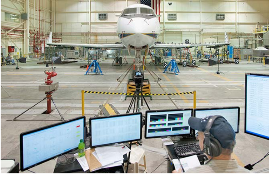
Aeronautical engineer William Lokos monitors a wing loading test of the NASA Gulfstream G-III SCRAT at the NASA Armstrong Flight Research Center's Loads Laboratory. (NASA)
