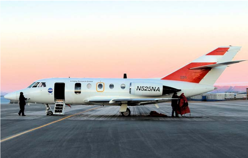
One of NASA's two ex-Coast Guard Dassault HU-25C Guardian Falcons used for a variety of earth sciences and other research missions. (NASA)
