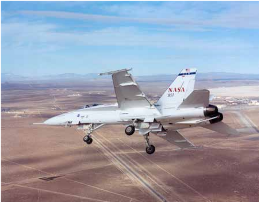
With landing gear and flaps down, NASA Dryden's Active Aeroelastic Wing F/A-18A research aircraft rolls toward final approach to the Edwards Air Force Base runway at the end of a test flight. (NASA)
