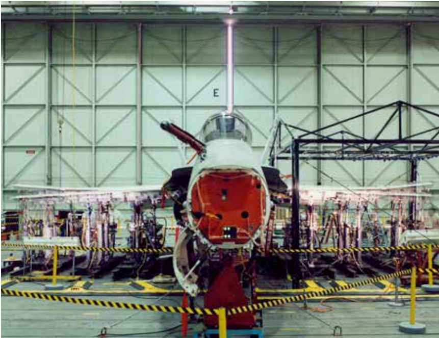
This multiple exposure emphasizes the wing deflections produced by test fixtures in the FLL. (NASA)
