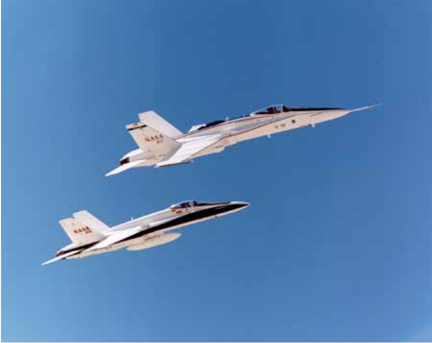
The AAW test bed flies formation with a production model F-18 serving as a chase plane. (NASA)
