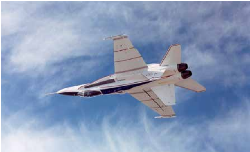
The AAW test bed flies upside down during a 360-degree aileron roll maneuver. (NASA)
