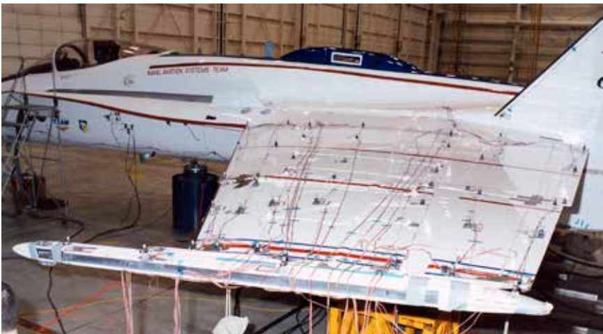
During ground vibration tests, the upper wing surfaces were covered with accelerometers and other sensors. The FDMS pod is visible atop the spine of the airplane above the wing. (NASA)
