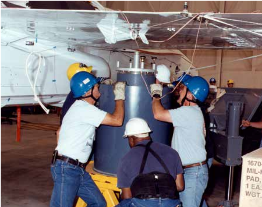
Loads Lab technicians including, from left, Dave Dennis, Freddy Graham, and Jeff Doughty position a support cylinder under the right wing of the AAW test aircraft prior to ground vibration testing. (NASA)
