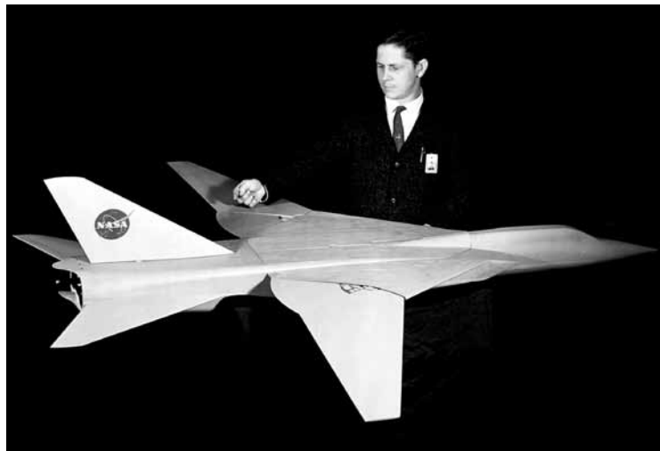
Free-flight model of outboard pivot variable-sweep model used in research studies at Langley. Conceived by researchers at the Langley 7- by 10-Foot High-Speed Tunnel, this configuration was tested across the speed range, including low-speed flight tests in the Full-Scale Tunnel.
