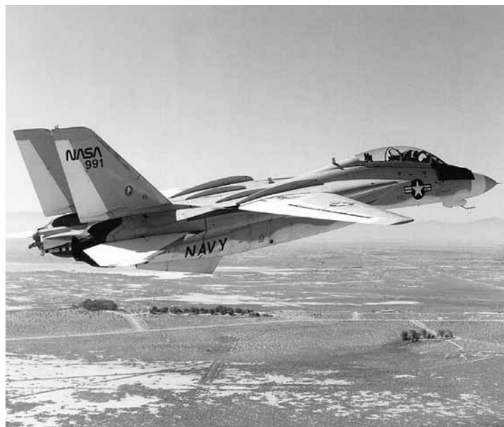
The F-14 used in the NASA–Grumman–Navy high-angle-of-attack program at NASA Dryden was equipped with an emergency spin recovery parachute system and foldout canards on the forward fuselage.
