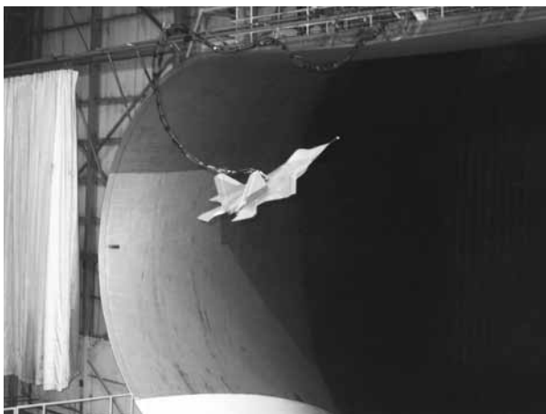
Free-flight evaluation of the dynamic stability and control of a powered model of the YF-22 fighter prototype at high angles of attack in the Langley Full-Scale Tunnel. The model was powered with compressed air ejectors and included thrust-vectoring engine nozzles and a nose boom equipped with angle-of-attack and sideslip vanes and sensors for implementation of critical flight control system elements of the full-scale aircraft. The outstanding behavior of the model at high angles of attack was subsequently verified by the airplane.
