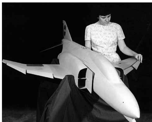
Free-flight tests of this model of the F-4 Phantom II in 1970 provided data for analysis of the wing rock and directional divergence exhibited by the configuration at high angles of attack. The test program also included demonstrations of the benefits of two-position fixed leading-edge slats, which were incorporated in later versions of the airplane.
