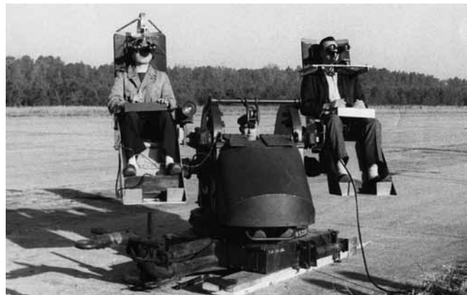
Ground control stations for pitch and roll-yaw pilots in early drop model tests. The crew consisted of a pitch pilot, a roll-yaw pilot, and a tracker operator. Binoculars were used for close-in views of the model during flight, and a tracking camera recorded motion pictures of the model's motions.
