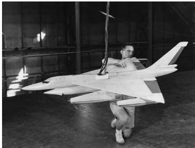
Free-flight model of the Convair XB-58 bomber is prepared for dynamic stability and control evaluations in the Full-Scale Tunnel.
