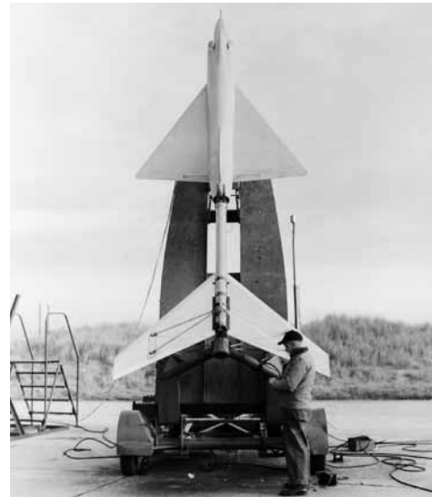
F-102 free-flight model is prepared for rocket launched flight at Wallops. Extensive flight testing of hundreds of rocket-boosted models occurred at Wallops during its NACA days. Note that the model has been modified with the wasp-waisted area rule concept conceived by Richard T. Whitcomb of Langley.
