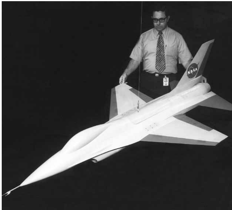
Free-flight tests of the YF-16 Lightweight Fighter Prototype demonstrated outstanding dynamic stability control characteristics within the design envelope. The results also clearly identified a severe directional divergence, which occurred for high angles of attack beyond achievable values limited by the flight control system.
