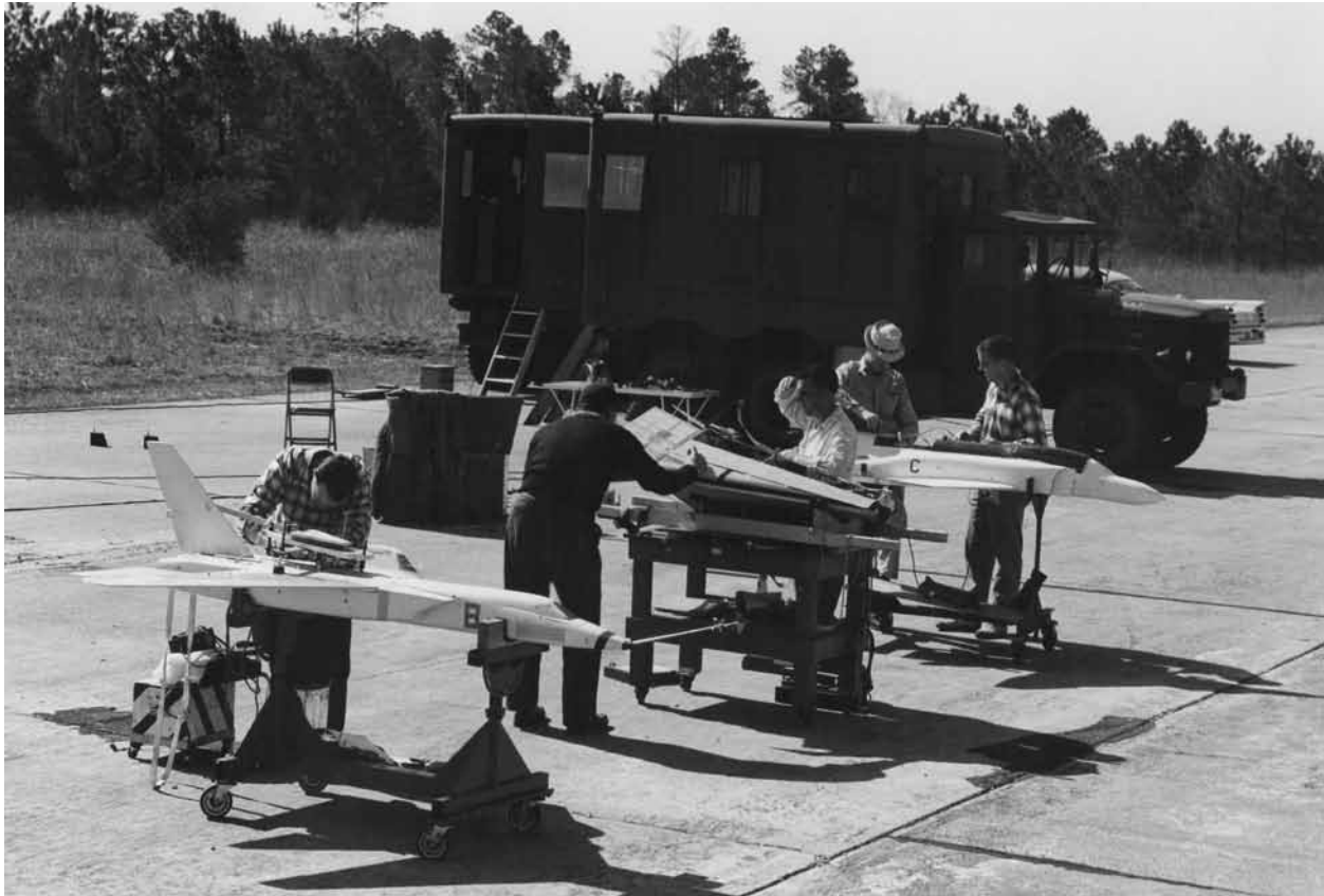
A busy day of testing for the drop-model test unit at West Point in 1960. Models being prepared for tests include models of, front to rear, the Navy A3J attack fighter, a NASA Langley hypersonic reentry shape, and the Navy F4H-1 fighter.
