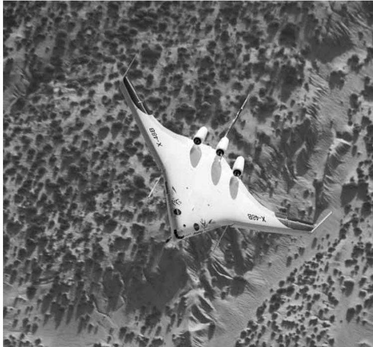
Free-flying dynamically scaled models have evolved from simple unpowered silk-span-covered balsa replicas to highly sophisticated miniature aircraft with advanced materials, propulsion units, control systems, and instrumentation. This model of the X-48B blended wing-body configuration is typical of the current state of the art in dynamic model technology.
