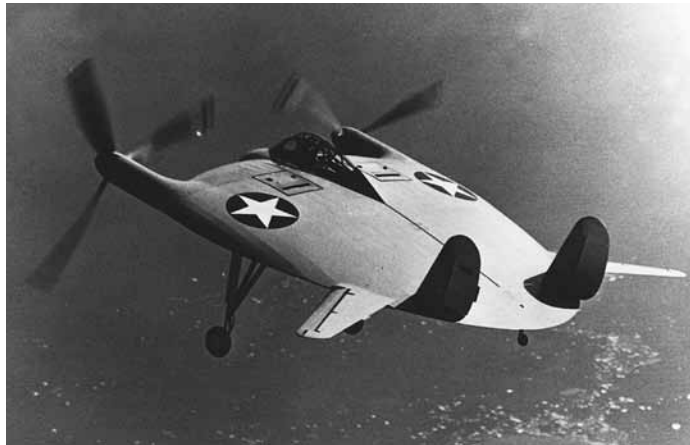
After modifications suggested by powered free-flight model tests at Langley, the V-173 full-scale aircraft was successfully flown and demonstrated outstanding short-field capability.
