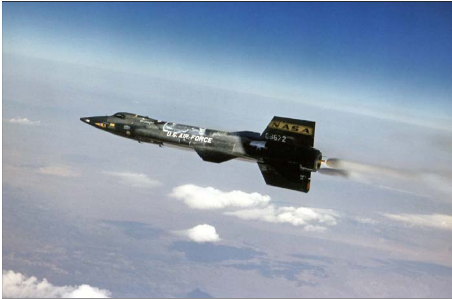
Figure 9-1. X-15 ship #3 (56-6672) is shown in flight over the desert in the 1960s. This spaceplane made 65 flights during the program, attaining a top speed of Mach 5.65 and a maximum altitude of 354,200 feet. (U.S. Air Force)
