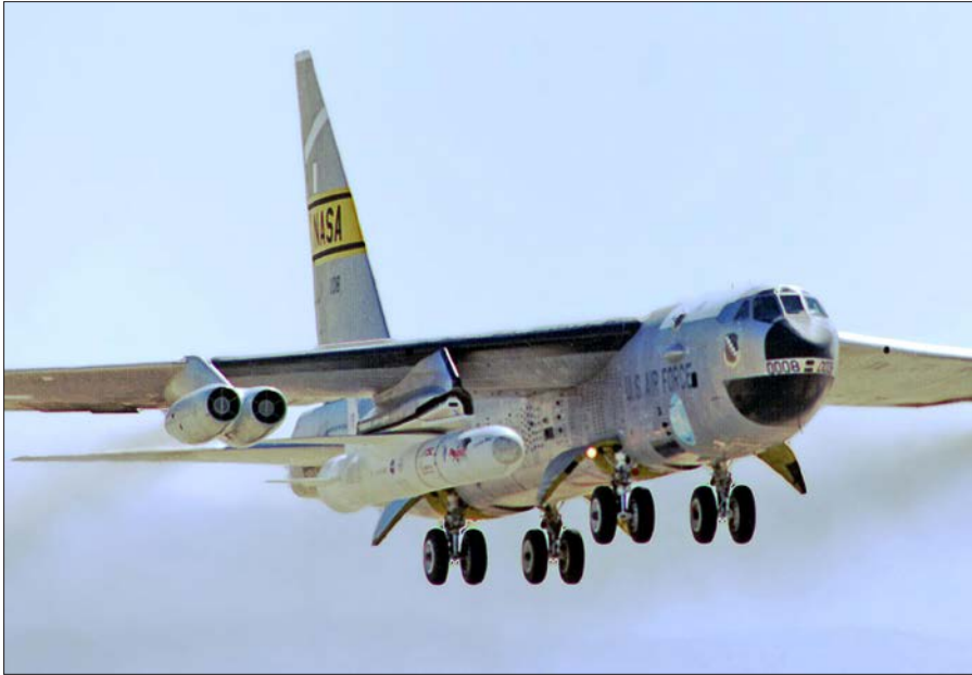
Figure 11-1. The Pegasus launcher was first developed by Orbital Sciences Corp. as a commercial launcher in the 1980s and had a lengthy career as an air-launched rocket delivering payloads to Earth orbit. Here NASA's B-52 mother ship takes off with the second Pegasus vehicle under its wing from the Dryden Flight Research Facility in July 1991. (NASA, 330365main_EC91-348-3_full)
