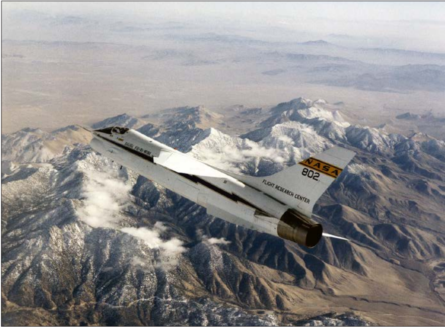
Figure 9-3. F-8 digital fly-by-wire (DFBW) aircraft in flight over snowcapped mountains. Although it is externally identical to a standard Navy F-8C, this aircraft had its control system replaced by an Apollo digital computer and other maneuvering electronics to document the superiority of this type of system. (NASA, ECN-3478)
