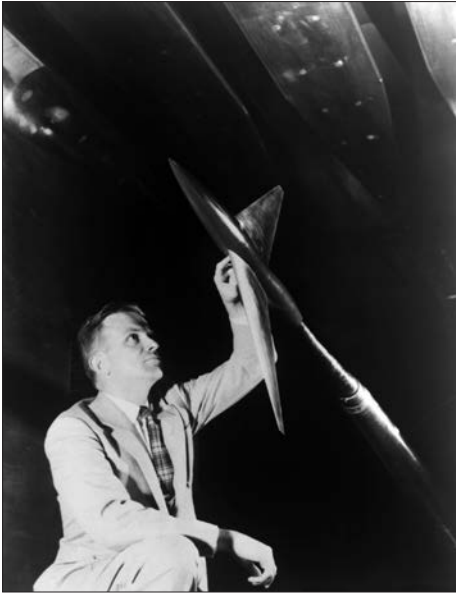
Figure 4-5. In April 1955, NACA engineer Richard Whitcomb examines a model designed according to principles of his transonic area rule in the Langley 8-foot High-Speed Wind Tunnel. (NASA, LRC-1954-B701_P-89119)
