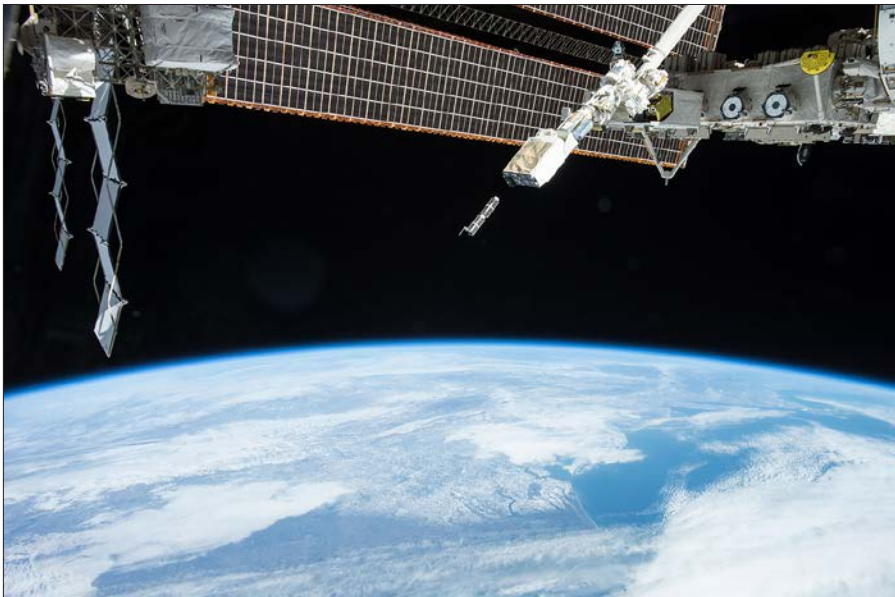
Figure 10-4. The Nanoracks CubeSat Deployer in operation on the ISS, 4 August 2017. (NASA, nanorack_deployment.jpg)
