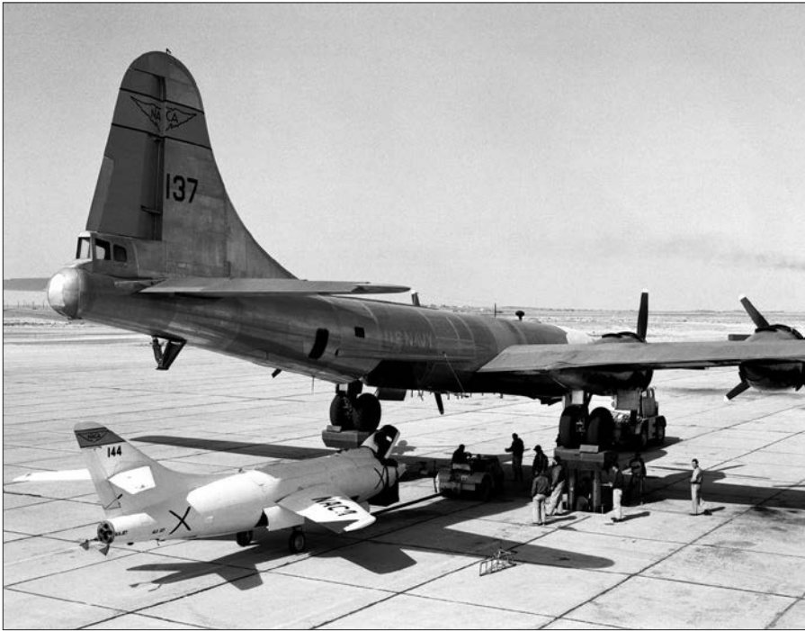
Figure 4-2. This 1953 image taken at the NACA's High-Speed Flight Research Station photograph shows the Douglas D-558-2 transonic aircraft being positioned under the B-29 mother ship prior to a research flight. (NASA, E-1013)
