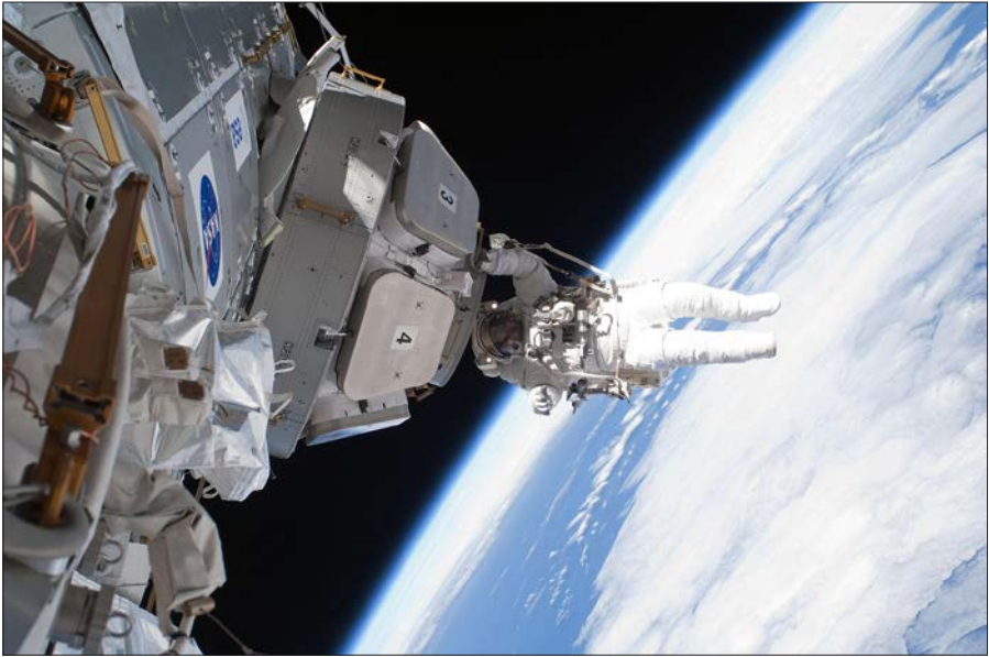
Figure 10-5. One of the last pieces of hardware to be assembled on the International Space Station, this cupola provides a window on the world. Floating just below the ISS, astronaut Nicholas Patrick puts some finishing touches on the newly installed cupola space windows in 2010. (NASA, 429583main_installingcupola_nasa_big)
