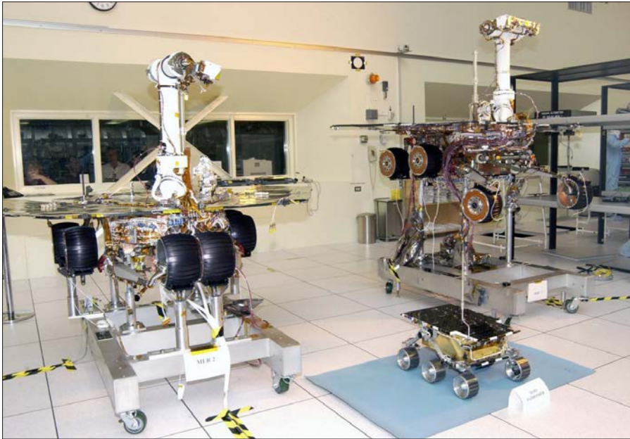
Figure 7-3. The twin rovers of the Mars Exploration Rover mission pose in 2003 just before launch to the Red Planet with their innovative predecessor, the flight spare of the Sojourner rover from NASA's 1997 Pathfinder mission. (NASA, PIA04422)
