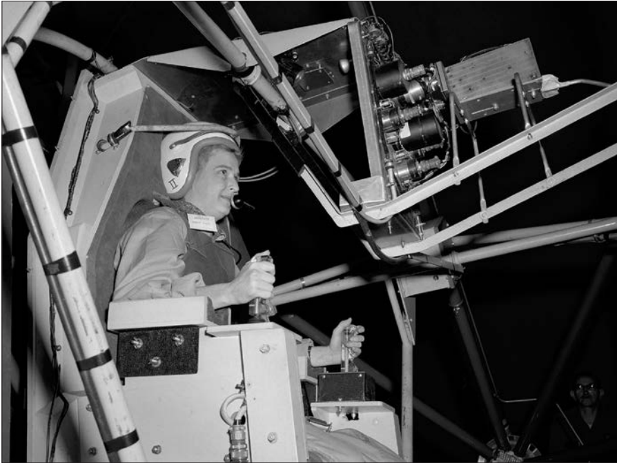
Figure 8-3. Jerrine Cobb, one of the women who underwent the same physical tests as the Mercury astronauts in the early 1960s, prepares to operate the Multi-Axis Space Test Inertia Facility (MASTIF) inside the Altitude Wind Tunnel at NASA's then-Lewis Research Center. (NASA, GRC-1960-C-53088)
