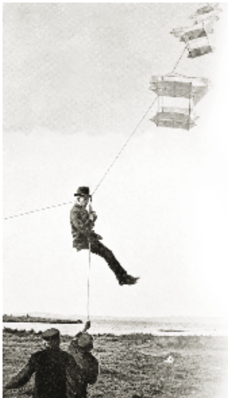
Roald Amundsen testing the so-called man-lifting kite in 1909. Perhaps the kite could be used for reconnaissance in the Polar Regions? In order to find out, Amundsen started trials in Horten. The results indicated that the kite was capable of lifting a person several hundreds of metres into the air. Then one day, lightning struck the steel wire of the kite. One of Amundsen's men was killed, and the trials were ended.
