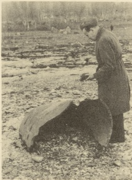
FRACTURED 12,000 lb. BOMB BODY ON FORESHORE
