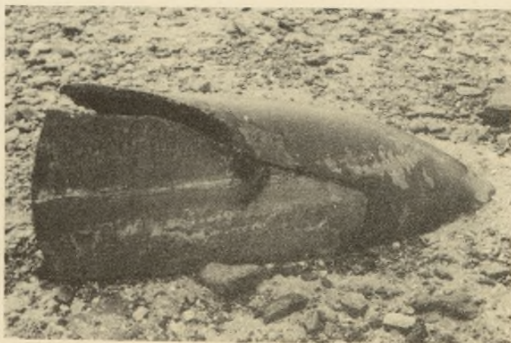
FRACTURED 12,000 lb. BOMB BODY ON FORESHORE
