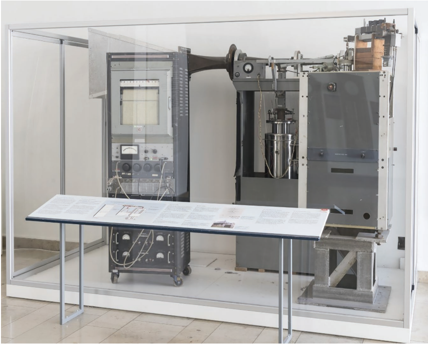
Figure 4.2 Deutsches Museum Collections Inv.Nr. L1992–3T1: Control box with maser and pre-amplifier
