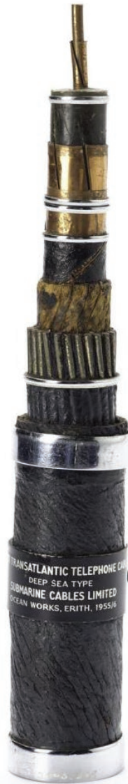
Figure 3.1 Cable sample, TAT-1 deep sea type, 1955. Made by Submarine Cables Ltd (NMS T2003.269), National Museums Scotland
