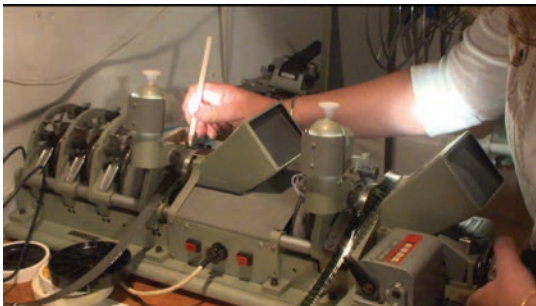
FIGURES 1.1–1.4 Television film and video editor Dawn Trotman demonstrating the use of an Acmade Pic-Sync during an ADAPT project reenactment exercise.
