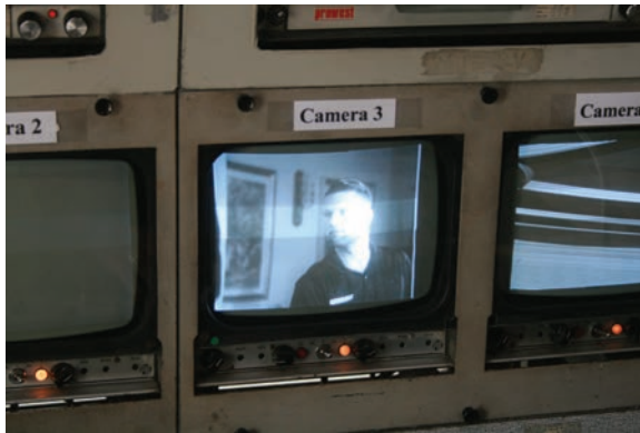
FIGURE 3.4 Images of a live darts match displayed on preview monitors inside ex-BBC outside broadcast truck North 3, during an ADAPT project reenactment exercise.
