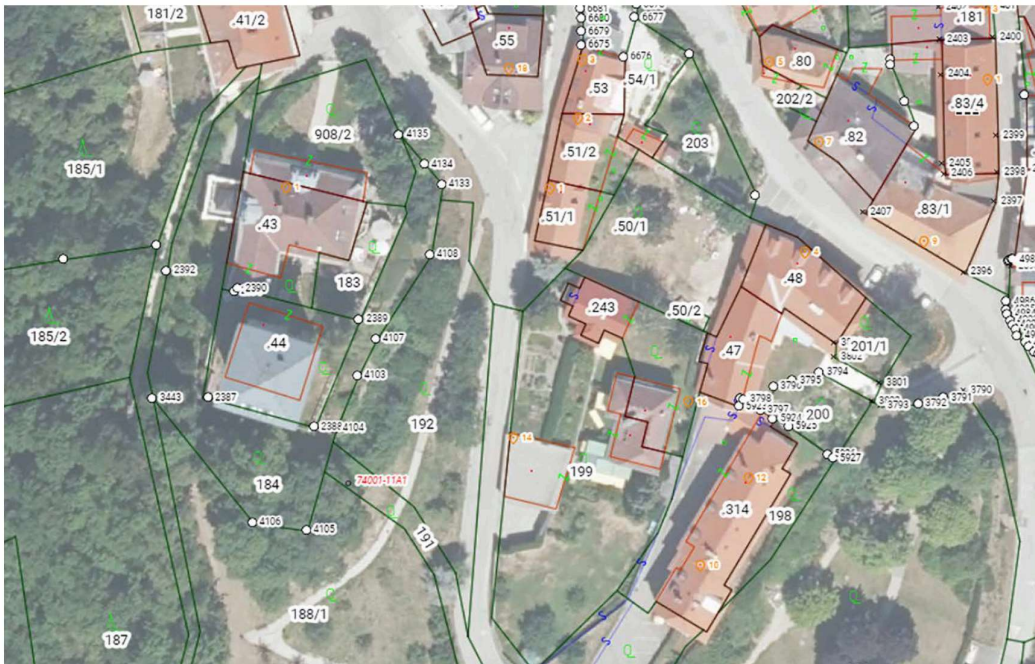
Figure 6. Cadastral Map Overlaid to Orthophoto (Source: www.kataster.bev.gv.at ).
